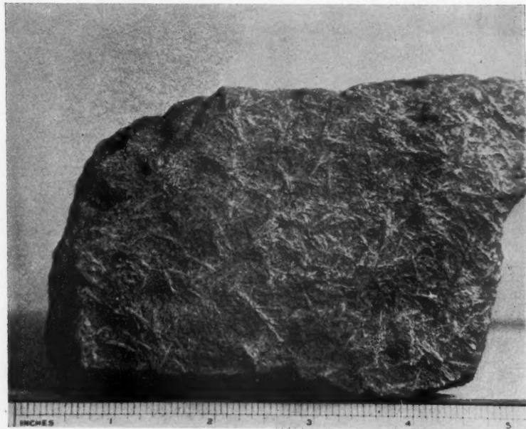
FIG. 2. Weathered surface of schist showing sillimanite with random orientation.
